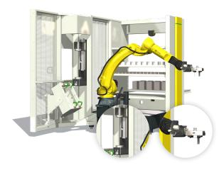
No more worries! Fully automated runs of six-sided milling operations. With the R-C2 | 6S version of the X35, they are within your reach. In a stable, fully automated process, for a high-mix/low-volume strategy. Thanks to a centric vice for the handling and a perfect take-over by the 6S station's second centric vice, all six sides can be completed automatically. Just one process step, and your parts are ready to ship!
